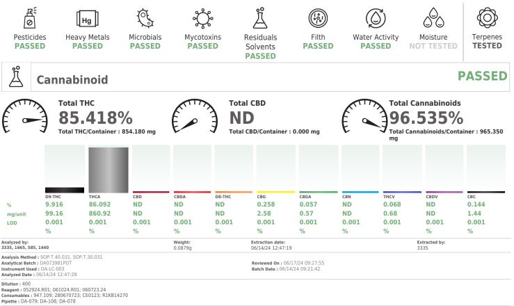
Full Spectrum cannabinoid analysis utilizing High Performance Liquid Chromatography with UV detection in accordance with F.S. Rule 64ER20-39
