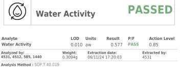
Reviewed On: 06/12/24 09:58:05 Analytical Batch : DA073865WAT Instrument Used : DA-028 Rotronic Hygropalm Batch Date : 06/11/24 12:50:41 Analyzed Date : 06/11/24 17:20:48 Dilution : N/A Reagent : 051624.01 Consumables : PS-14 Pipette : N/A
