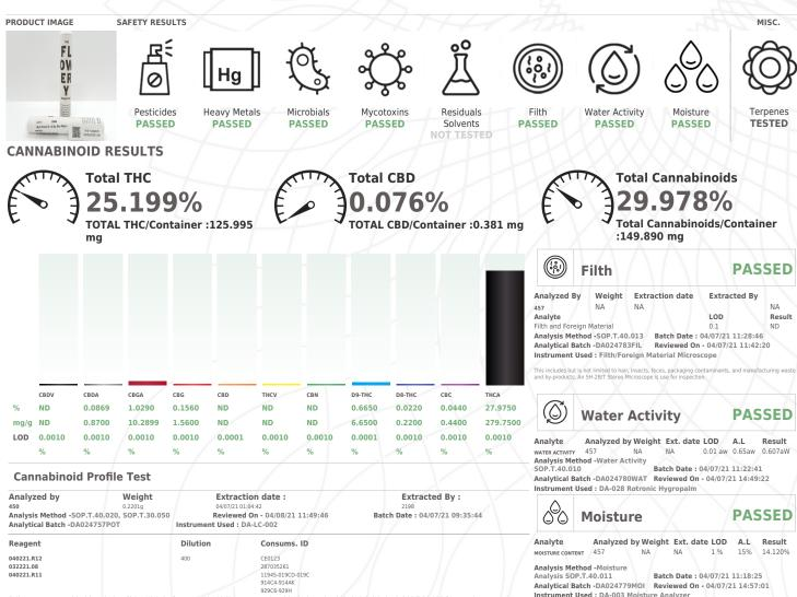
Full spectrum cannabinoid analysis utilizing High Performance Liquid Chromatography with UV detection (HPLC-UV). (Method: SOP.T.30.050 for sample prep and Shimadzu High Sensitivity Method SOP.T.40.020 for analysis. LOQ for all cannabinoids is 1 mg/L).
